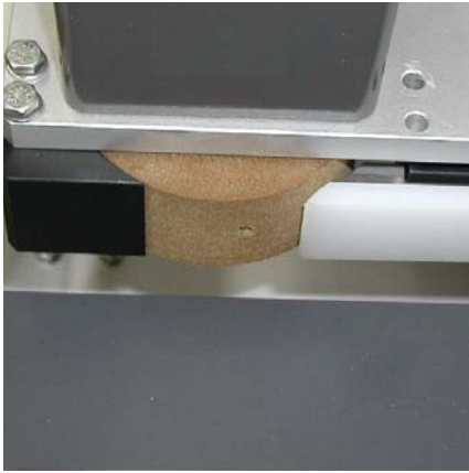
Roller-type separator and roller prism of model HERMA 152 C Prisma, easily adjustable
