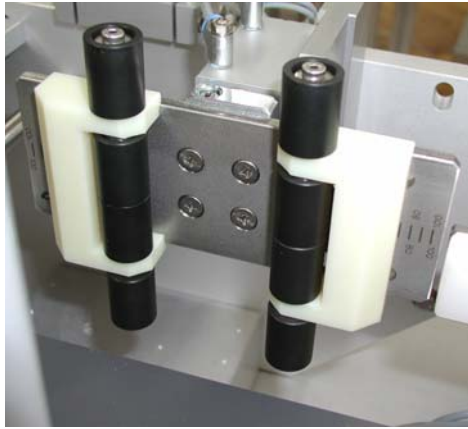
Roller-type separator and roller prism of model HERMA 152 C Prisma, easily adjustable
